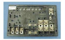
Insert molding circuit board
